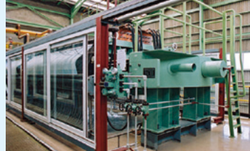
Ion-exchange membrane chlor-alkali electrolysis process
