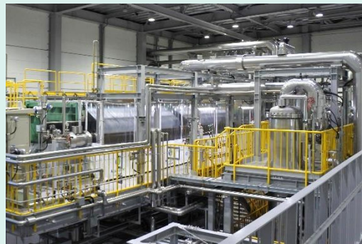
10 MW-class alkaline water electrolysis plant
