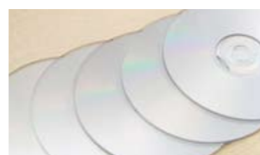
CDs made of polycarbonate
