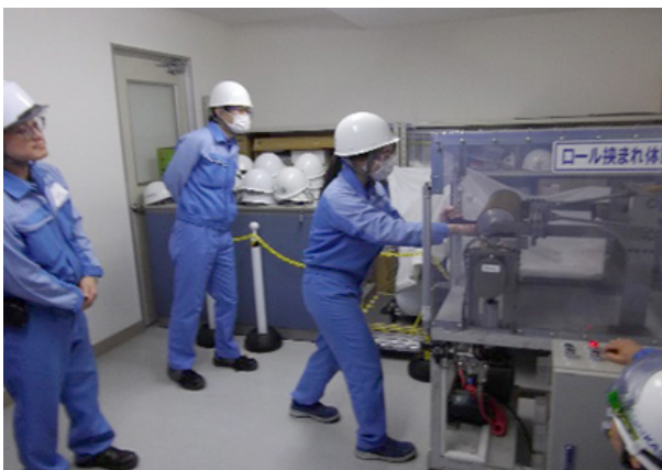
Simulated experience of being caught in a rotary valve (Kawasaki Works)
